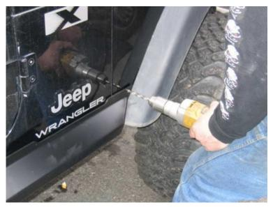
3. Using a 5/16" drill bit, drill out all marked holes through into the tub.
