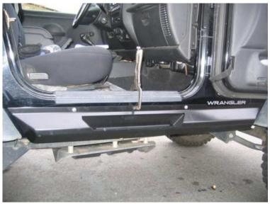
1. With rocker skid held in place, transfer and mark all holes along the body for drilling. Also transfer the holes on the underside of the tub as well. The TJRP-P has 3 underneath, the LJRP-P has 4 underneath.
