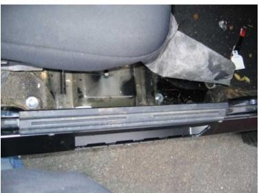
4. Install supplied bolts through the side of the body and up through the tub. Secure on the backside using flat washer and lock nut. Loosely start all bolts before tightening them all down
